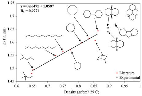
Figure 2. Refractive index (193 nm) of cycloalkenes and noncycloalkenes as a function of the density.
