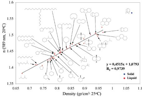
Figure 1. Refractive index (d line) vs density of alkanes and cycloalkanes at room temperature.
