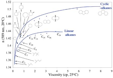
Figure 3. Refractive index (d line) vs viscosity of liquid alkanes and cycloalkanes at room temperature.
