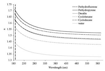
Figure 4. Refractive index vs wavelength of polycycloalkanes.
