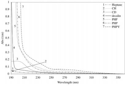
Figure 7. Absorption spectra of cycloalkanes and polycycloalkanes used in this study.
