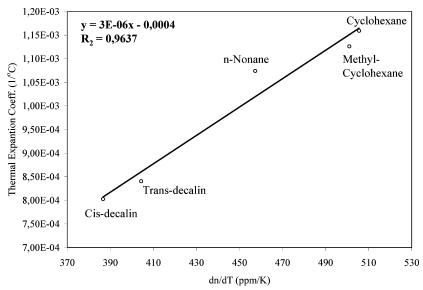
Figure 6. Relationship between thermal expansion coefficient and the temperature dispersion of the refractive index at 589 nm of some cycloalkanes.
